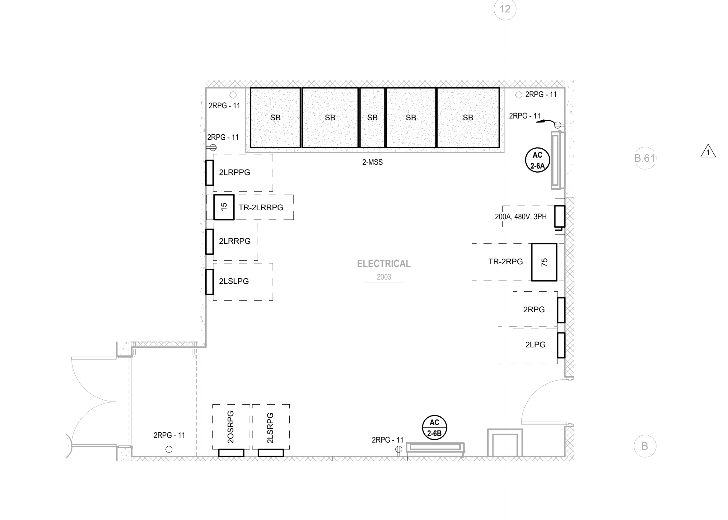
1 BUILDING NO.2 - ENLARGED ELECTRICAL ROOM 2003 E-303 SCALE: 1/4" = 1'-0"
